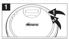
Press the PLAY/PAUSE (▶Ⅱ)/POWER ON/▲ button ① to turn the unit on. To turn the unit off, press the STOP (■)/POWER OFF/▼ button ②. The unit will automatically shut off if stopped (CD Standby) for one minute.
